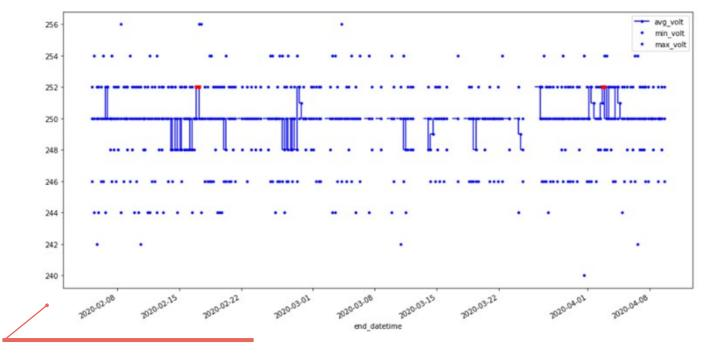
Instances of average voltage exceeding nominal voltage and maximum value over a set threshold
